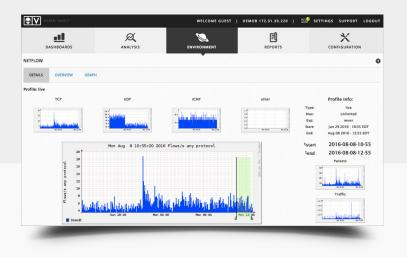
**NetFlow Analysis** captures metadata from the TCP/IP stream and analyzes the protocols and calculates the bandwidth used by each protocol.
