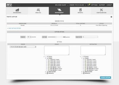
**Network Traffic Capture** allows for forensic storage of the packet stream so that detailed inspection can be performed if necessary.
